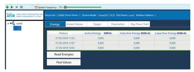
5 - when the device is selected consumption data can be seen from the Reports menu. Time Range should be selected in the window that opens.
